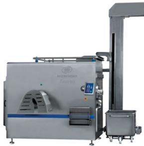
TAURUS W-200B angle grinder is designed for grinding blocks of meat frozen down to  $-20^{\circ}\text{C}$  and for other processing operations according to the used equipment. The device has a special design to grind the entire blocks of frozen meat. The angle grinder ensures a high quality of ground meat.
